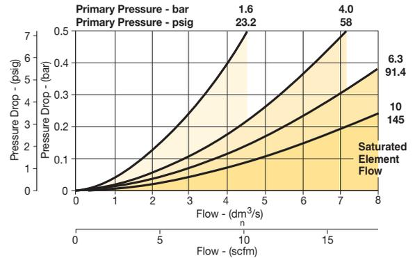
P31 - 0.01 micron flow Coalescing Filter
