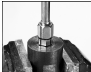
Fig. C15 — Fully tightened positioned with displaced mark
