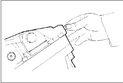
Position of setting piston, which also serves as a limitation for min. displacement. (First remove the plug).
