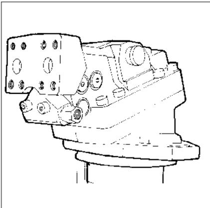
To adjust setting-time, remove the pilot valve cover.
