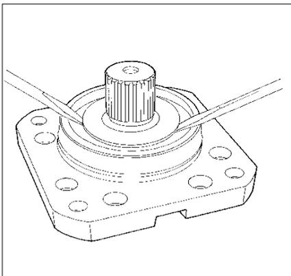
Pull out the seal carrier. Remove the old seal ring, install a new seal ring and push the carrier back into the V12 motor.
