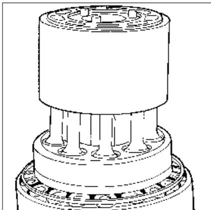
Install pistons, joint with support and rollers and cylinder barrel on the shaft.
