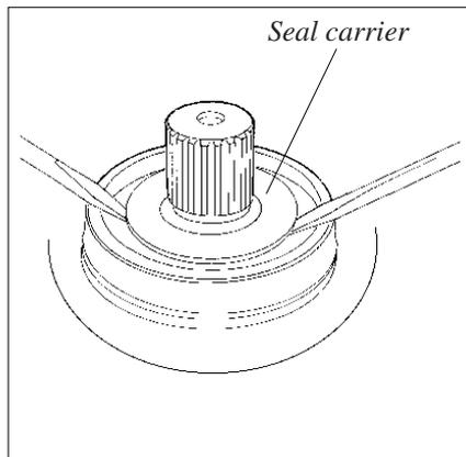
Remove the retaining ring and pull out the seal carrier.
