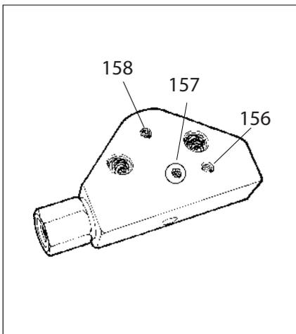
The setting times for T12 is changed by installing different nozzles in the pilot valve cover. Nozzle position 157 reduces setting time to booth max. and min. displacement. Nozzle position 156 reduces setting time to max. displacement. Nozzle position 158 reduces setting time to min. displacement.
