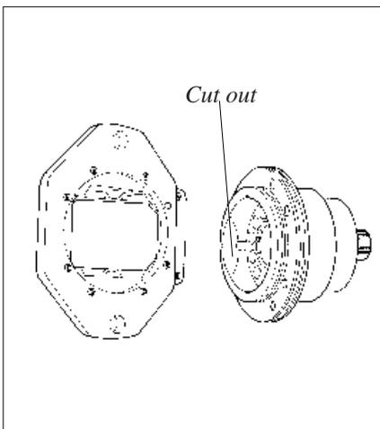
Install the bearing housing. In the cartridge version bearing housing there is a cut out for the pistons at max. angle setting. The bearing housing and the flange cannot be assembled wrongly as there is an irregularity in the pitch for the holding screws.
