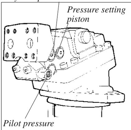
Note, 156 is also the drain connection from the pilot valve, why too small nozzle in this position might influence the function of the pilot valve (the valve might stop operating, specially for low pilot pressure).
