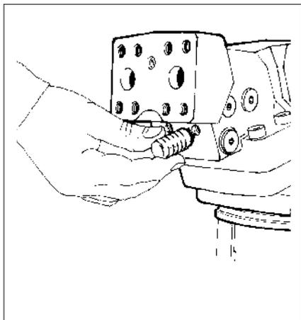
Position of setting piston, which also serves as a limitation for max. displacement. (First remove the pilot valve cover).
