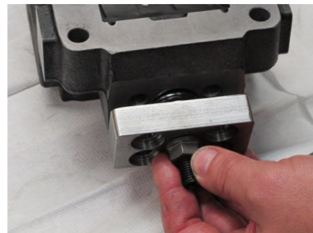
39. Assemble the cover assy. Make sure not to damage the O-ring.
