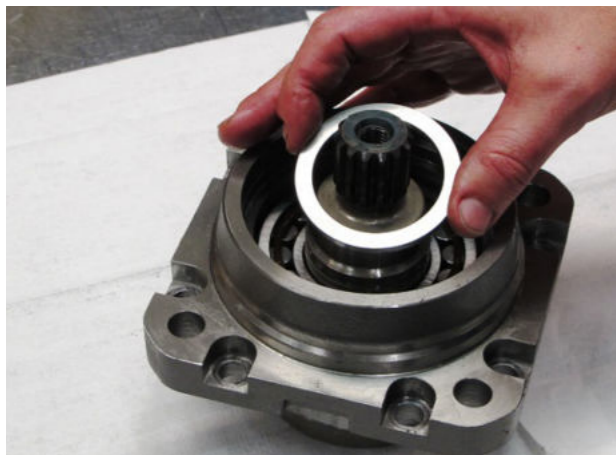
3. Assemble the bearing ring with the text downwards.
