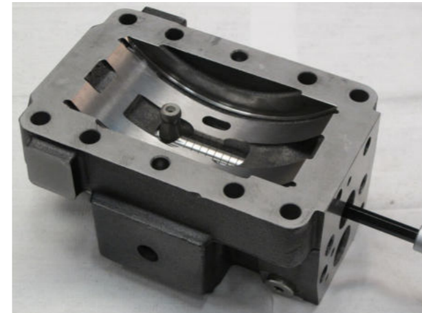
26. Torque the set screw to 26±6 Nm. Move the companion pin back and forward to make sure it moves smooth.
