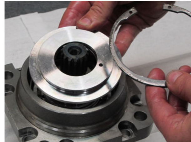
8. Assemble the seal carrier with shaft seal and the retaining ring. Make sure it is all the way into the groove.
