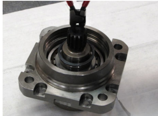
5. Assemble the retaining ring. Make sure it is all the way into the groove. Check the pre-load of the bearings, not too tight and no back-lash.
