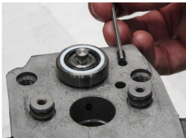
36. Assemble the nozzles and torque them to 1,2 \pm 0,2 Nm.
