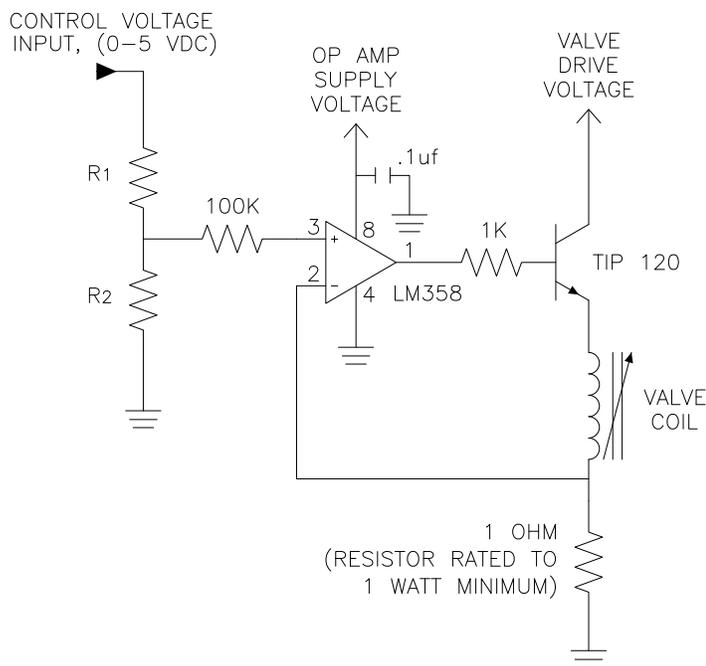
This simple current driver circuit draws only 1 mA at the input control (0-5VDC) and provides control for any Lone Wolf configuration regardless of valve voltage or resistance.
