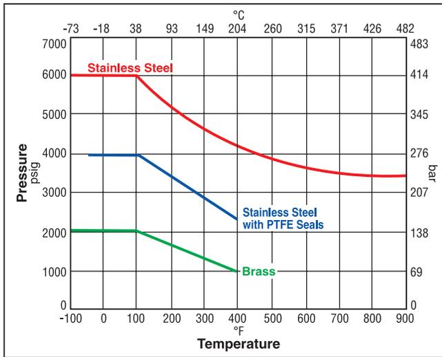
**Note:** This Pressure versus Temperature chart reflects the maximum temperature range of indicated body materials.
