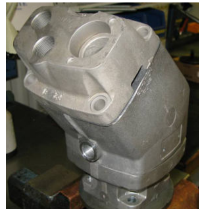
The number and thickness of gaskets determines the backlash
