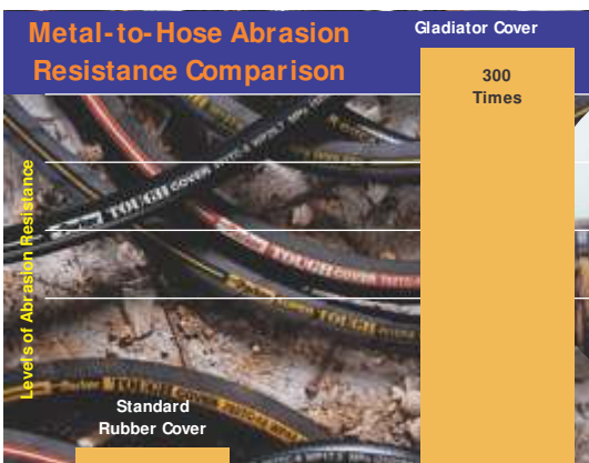
Results from the ISO 6945 metal to hose abrasion test show that Gladiator cover hose offer significantly greater abrasion resistance than standard rubber cover hose.
