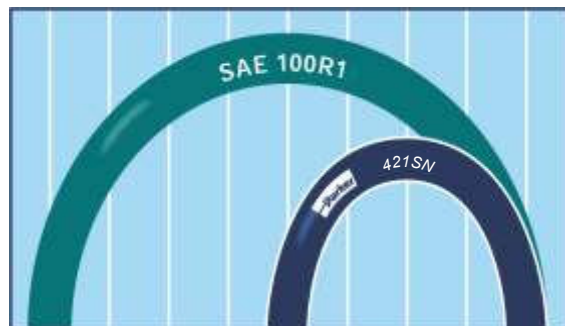
301SN / 421SN hoses has half the minimum bend radius of DIN 2SN / 1SN hoses.
