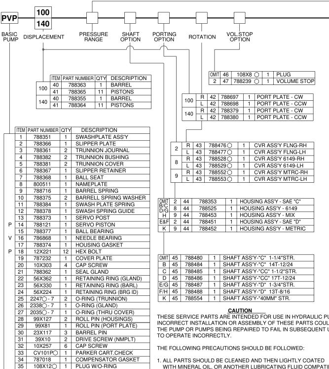
THESE SERVICE PARTS ARE INTENDED FOR USE IN HYDRAULIC PUMPS. INCORRECT INSTALLATION OR ASSEMBLY OF THESE PARTS COULD CAUSE THE PUMP OR PUMPS BEING REPAIRED TO FAIL IN SUBSEQUENT USE, OR
