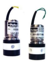
The 2-Way & 3-Way inert Series 1 & 2 valves have been designed for systems where chemical compatibility is most important. The wetted path is isolated from the solenoid and only PTFE and borosilicate glass are in contact with the media passing through the valve. Low internal volume and fast response time ensure repeatable, accurate volumes. Valves will actuate without any pressure or vacuum applied.
