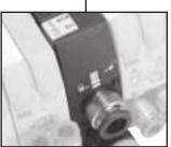
**#1 Open, #3 Blocked** #1 Port connected to valves on the right and the left.
